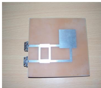
Figure 15 Fabricated Patch Antenna
